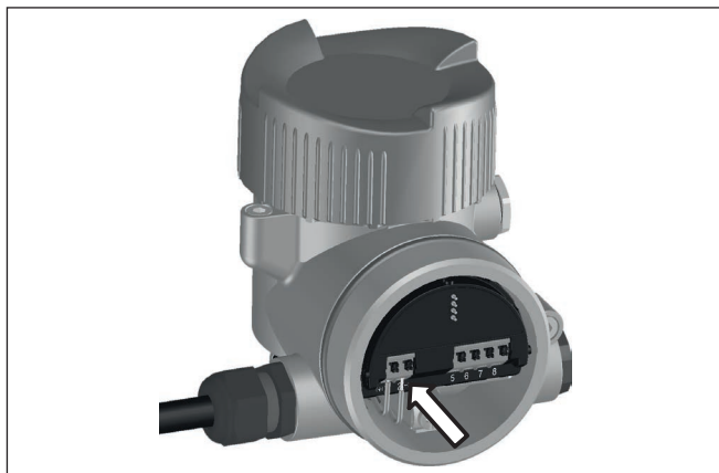
Fig. 11: Connection steps 5 and 6 - Double chamber housing
